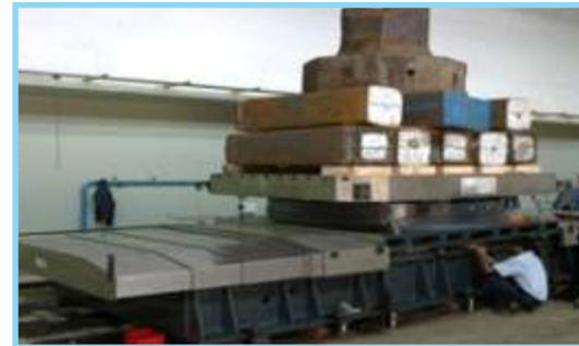
PERFORMANCE TESTING CNC ROTARY TABLE (40 Ton)
